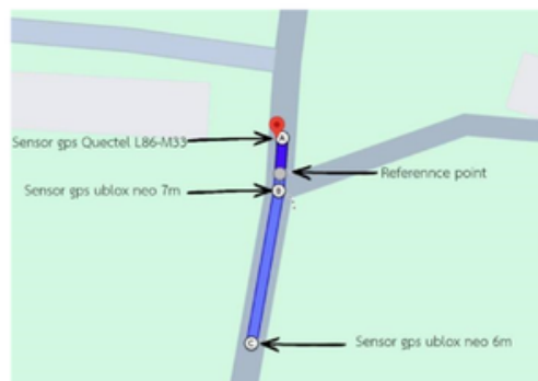
Figure 3. Comparison of coordinate positions from the three GPS sensor models against the reference position.
